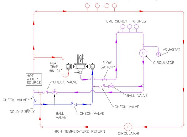
\* FLOW SWITCH MUST BE LEVEL AND IN CORRECT DIRECTION
