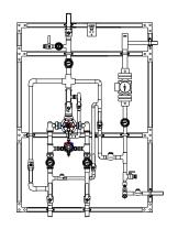
**HBP** High temperature by-pass flush with locking ball valve
