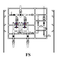
Megatron® with separate legs to the floor (shipped loose), attaches to channel of existing megatron to support the unit without hangers.
