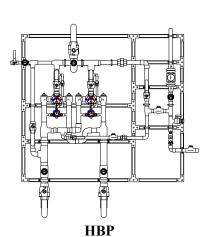
High temperature by-pass flush with locking ball valve
