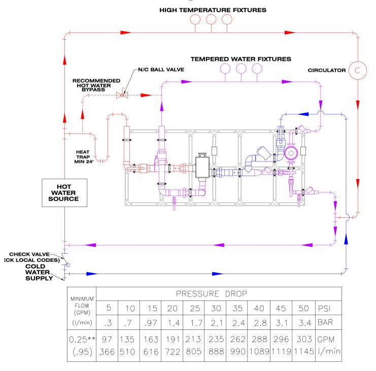
NOTE: Flowrates will vary depending on existing field conditions. Leonard Valve Company always recommends using CASPAK® sizing software for proper valve sizing and model number applications.
