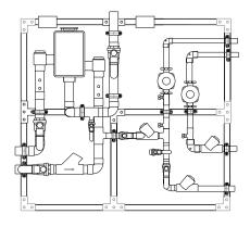
2 PUMPS H High temperature loop recirculation pump
