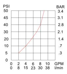
**CAUTION!** All thermostatic water mixing valves have limitations. They will NOT provide the desired accuracy outside of their flow capacity range. Consult the Flow Capacity Chart and DO NOT OVERSIZE. Minimum flow must be no less than as indicated.
