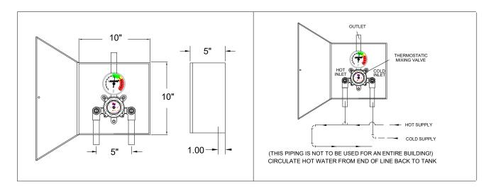
CAUTION! It may be necessary to recirculate the tempered water to the eye/face wash should the piping be exposed to excessive hot or cold conditions. Consult factory for proper piping.
