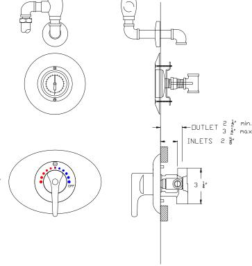
All Leonard Model 7600 Thermostatic Shower Valves have limitations. Please keep in mind that per the ASSE 1016-2011 Performance Standard, Harmonized along with ASME and CSA, it dictates inlet conditions of equal pressures, 45 PSI on both Hot and Cold Inlets, in addition to a Hot supply temperature range of 140 deg F- 180 deg F. Significant deviations from those conditions stated above will alter performance expectations.
