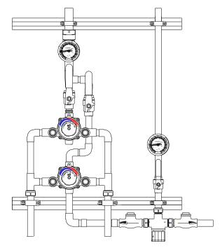
Valve assembly is certified to meet Low-Lead requirements of wetted surface area containing less than 0.25% lead by weight. All other fittings and components, the sum total of which comprise the wetted surface of this product contain less than one quarter of one percent of lead by weight.
