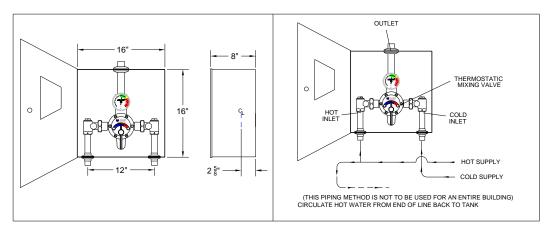
CAUTION! It may be necessary to recirculate the tempered water to the emergency shower should the piping be exposed to excessive hot or cold conditions. Consult factory for proper piping.
