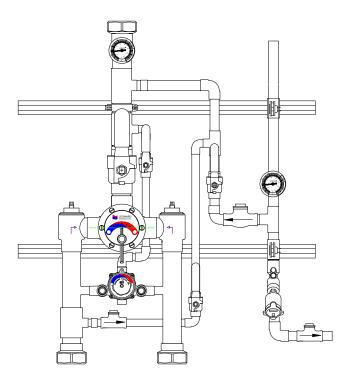
Valve assembly is certified to meet Low-Lead requirements of wetted surface area containing less than 0.25% lead by weight. All other fittings and components, the sum total of which comprise the wetted surface of this product contain less than one quarter of one percent of lead by weight.
