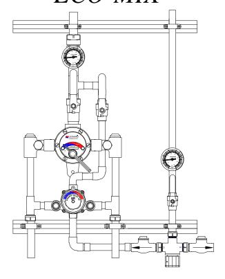
Valve assembly is certified to meet Low-Lead requirements of wetted surface area containing less than 0.25% lead by weight. All other fittings and components, the sum total of which comprise the wetted surface of this product contain less than one quarter of one percent of lead by weight.
