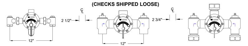
Note: The bottom port has been removed and is no longer available. If you are replacing an old valve that has the recirculation piped into the bottom port you will need to re-pipe the return. Please see Leonard's Piping Method #5.
