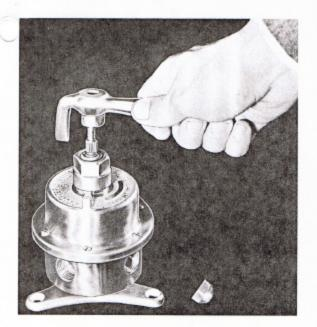
IF THE VALVE DELIVERS WATER TOO HOT (OR TOO COOL) WHEN POINTER IS IN "HOT" POSITION the Pointer may have been changed from its original position on the Pointer Rod. This would alter the high temperature limit.
