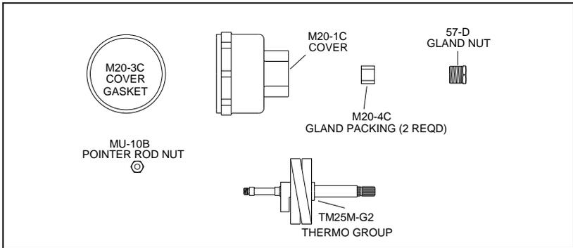
**NOTE:** AFTER INSTALLING NEW PARTS IT WILL BE NECESSARY TO RESET THE ADJUSTABLE HIGH TEMPERATURE LIMIT STOP (SEE PAGE 2).
