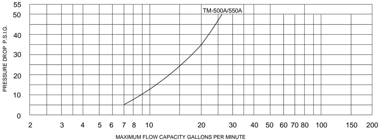
**CAUTION!** All thermostatic water mixing valves have limitations. They will not provide the desired accuracy outside of their flow capacity range. Consult the capacity chart and **DO NOT OVERSIZE**. Minimum flow must be no less than shown below.
