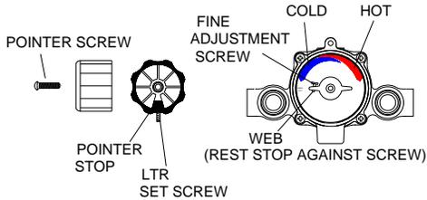
1. Loosen LTR Set Screw, remove POINTER SCREW.
