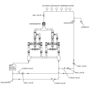
**CAUTION!** All thermostatic water mixing valves have limitations. They will NOT provide the desired accuracy outside of their flow capacity range. Consult the Flow Capacity Chart and DO NOT OVERSIZE. Minimum flow must be no less than as indicated.
