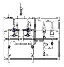
2 PUMPS R Redundant recirculation pump
