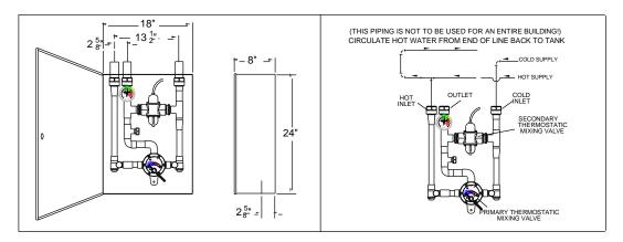
CAUTION! It may be necessary to recirculate the tempered water to the emergency shower should the piping be exposed to excessive hot or cold conditions. Consult factory for proper piping.
