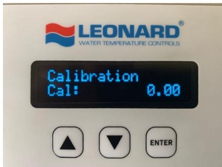
This Calibration Screen is used if the outlet valve temperature display differs significantly from a downstream temperature measurement value. It is a way to OFFSET the outlet temperature in order to agree with another temperature measurement value. Press **ENTER** to adjust Cal value, it will flash. Use ▲ ▼ buttons to adjust Cal value (+/-) in order to agree with other values. Press **ENTER** to save the Cal value. If Calibration is not needed, Press the ▼ arrow to advance to the next screen.
