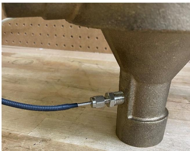
INSTALLATION OF COMPRESSION FITTING AND OUTLET RTD PROBE ON NEUTRON VALVE BODY
