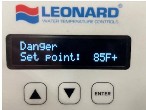
This Error indicates that the outlet temperature leaving the valve is outside of the tepid water temperature range, 65-95°F. The message will alternate with the Current Outlet Temperature.
