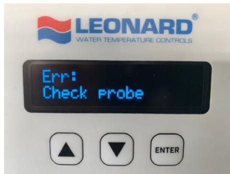
This Error indicates that the RTD Temperature Probe installed in the valve outlet is either disconnected from the Control Box or the wires are broken and it is in need of replacement. Please verify 3 wire connector on left side of control box is firmly engaged and verify that wires are continuous to the probe end. Replace if necessary. See Page 10 for details.
