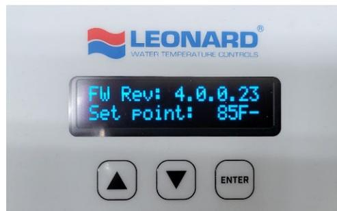
Pressing ▼ 2 times displays **FW Rev: X.X.X.X**
