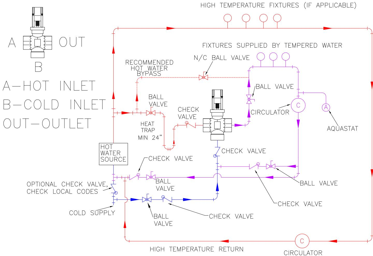
**Inlet Check Valves are required to prevent cross flow on all models**
