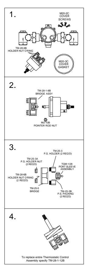
NOTE: AFTER INSTALLING NEW PARTS IT WILL BE NECESSARY TO RESET THE ADJUSTABLE HIGH TEMPERATURE LIMIT STOP (SEE PAGE 2).
