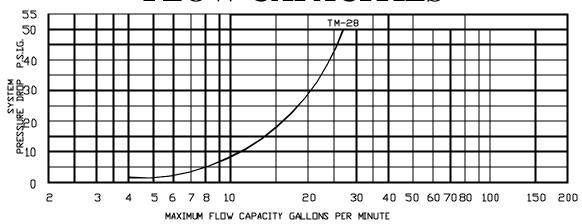
**CAUTION!** All thermostatic water mixing valves have limitations. They will not provide the desired accuracy outside of their flow capacity range. Consult the capacity chart.
