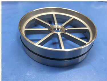
6. Inspect the shuttle and clean any sediment or debris that has built up. Replace O-ring if necessary.
