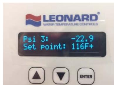
This is an indication of the actual measured value of pressure (PSI) on pressure sensor 3 (P3) if the Nucleus is so equipped with the optional Pressure Sensor (P3).
