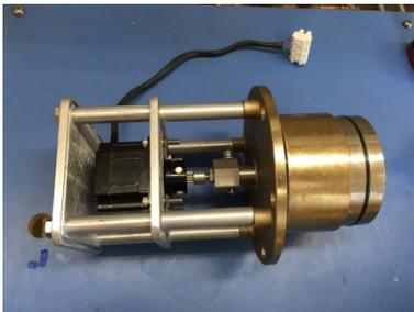
4. Remove complete cover assembly. Do not remove motor assembly at this time.
