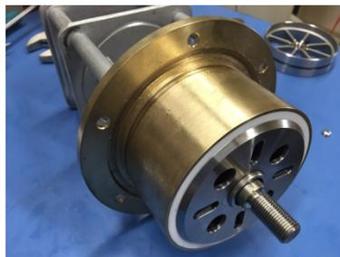
7. Inspect and clean all surfaces of the cover. Replace cover O-rings if necessary.
