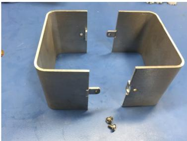
3. Remove the aluminum guarding and cover screws from cover assembly.
