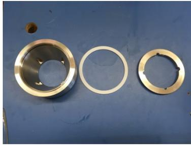
9. Remove sleeve assembly from valve body and clean all surfaces. Replace O-ring on bottom of part if damaged or worn. If necessary, disassemble the sleeve to install replacement Teflon® disk.
