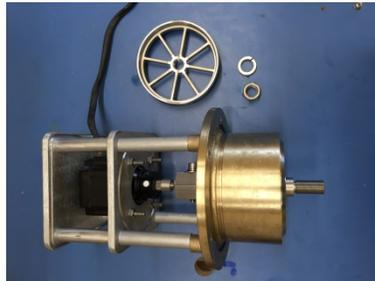
5. Turn the cover assembly on its side. While securing the hex-coupling under the motor mounting plate, remove the nut, lock washer and shuttle from the control stem.
