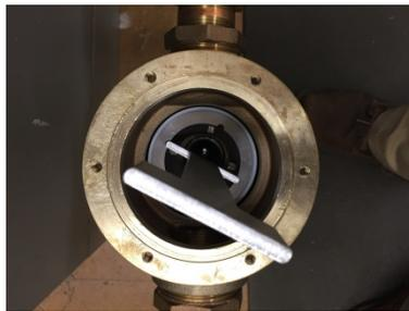
Loosen Sleeve Locking Nut
